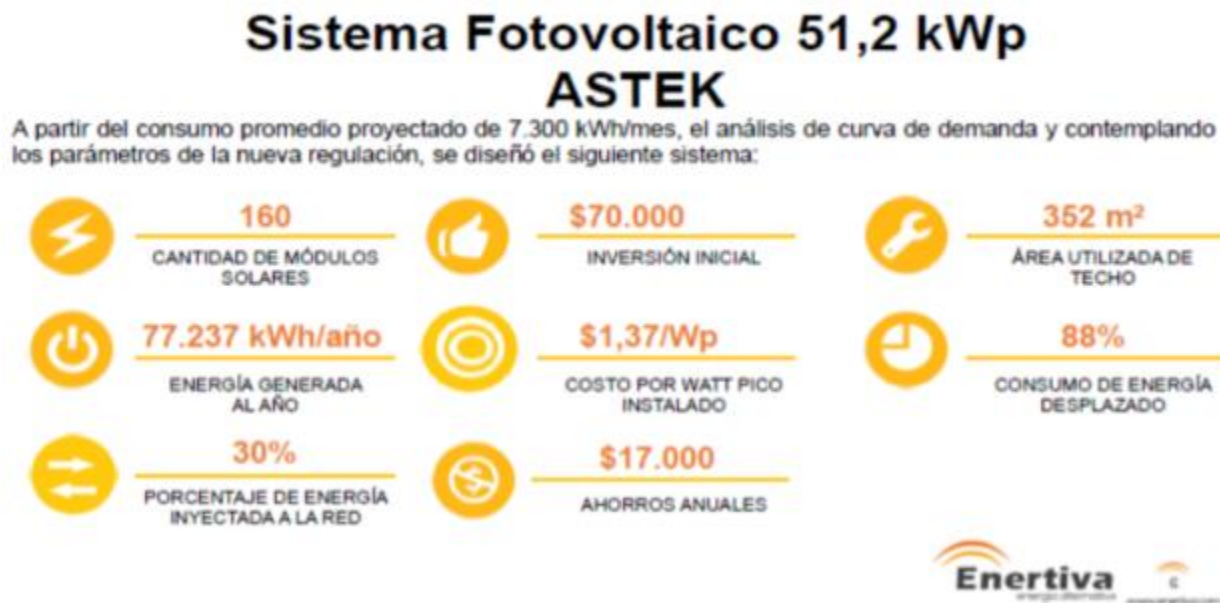
Figure 8: Astek solar panel system details
