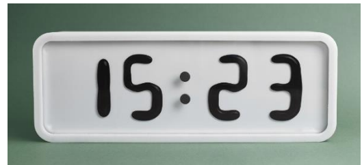
Figure 7. Ferrofluid Clock; Magnetic fluid behind glass with an array of magnetic coils form various numbers.
