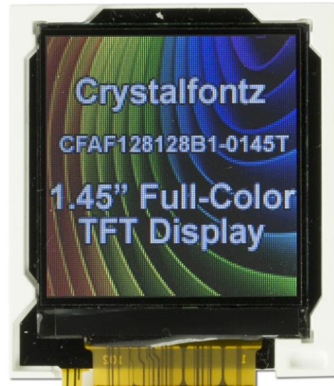
Figure 5. Crystalfontz 1.45" Full-Color TFT Display. This could be a single bead in the Perlenspiel display Source: IIR
