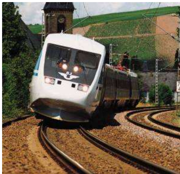
Figure 1: Swedish X2000 tilting train, top speed 200km/h or 125mph [2]
