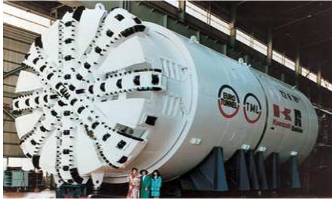
Figure 7 One of the world's largest TBMs with a diameter of 14m.
