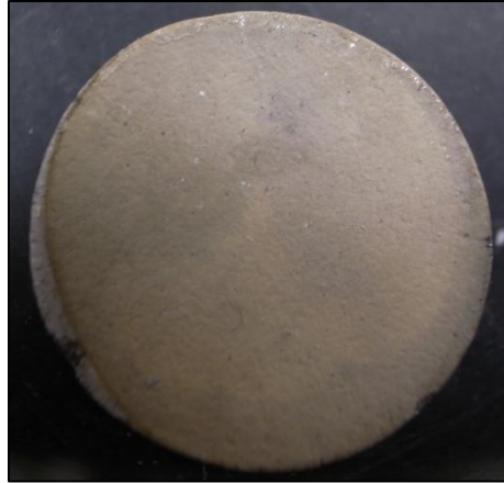
Figure 23: SiC porous support that has been plated with palladium
