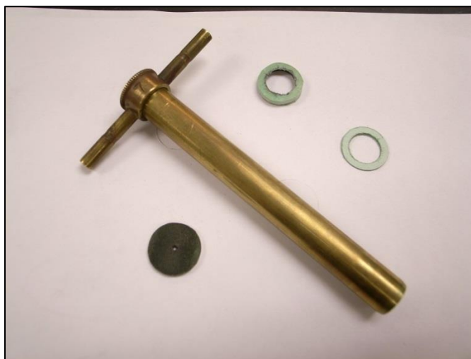
Figure 31: The Two Gaskets (top-right), the NiO Support (bottom-left), and the Hand Cutter Used to Make the Gaskets (center)
