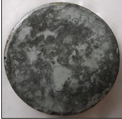
Figure 39: SiC chip with some of its plating ripped off
