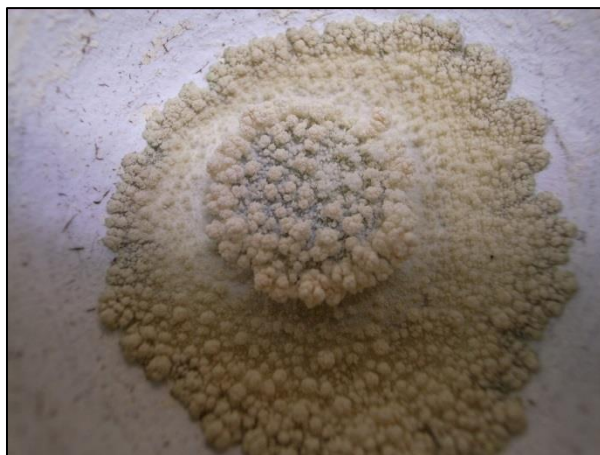
Figure 38: SiC chip covered in potassium carbonate crystals
