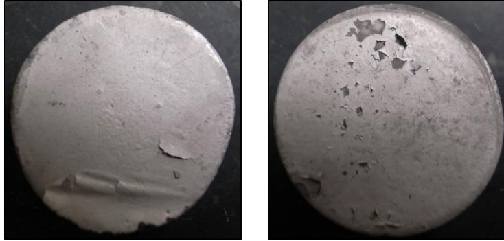
Figure 40: a) and b) Peeling-off plating due to annealing
