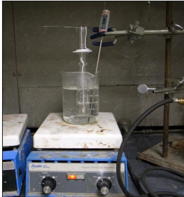
Figure 22: Plating Process Setup
