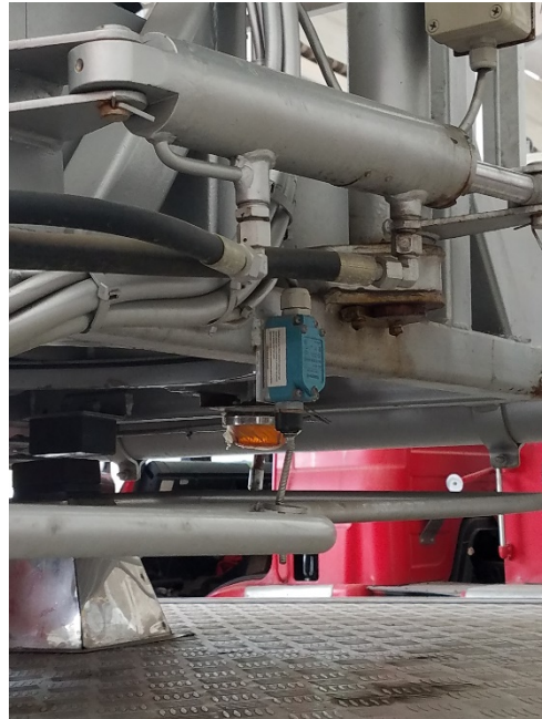
Figure 6 Example of Simple Switches
