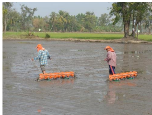
Figure 16: Operation of Rice Sowing Machine
