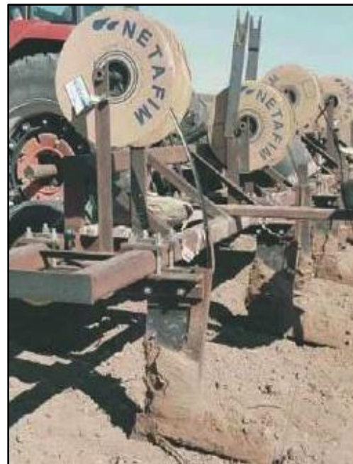
Figure 10: Drip line injector
