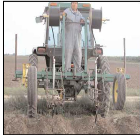
Figure 9: A shank making drip lines
