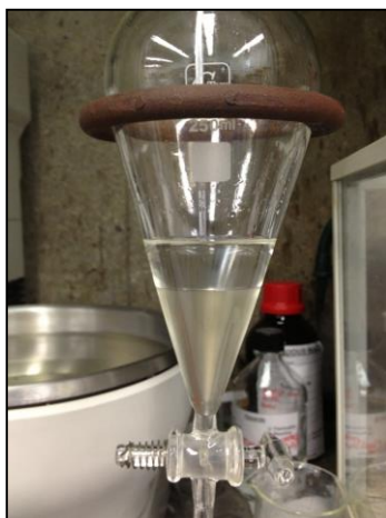
Figure 16: Organic and Aqueous phases in the separatory funnel
