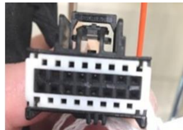
Figure 26: On the left is the K74 Human Machine Interface Control Module as pictured in the 2014 documentation, which has 16 pins in two rows of eight. On the right is the same connector on the 2015 harness.
