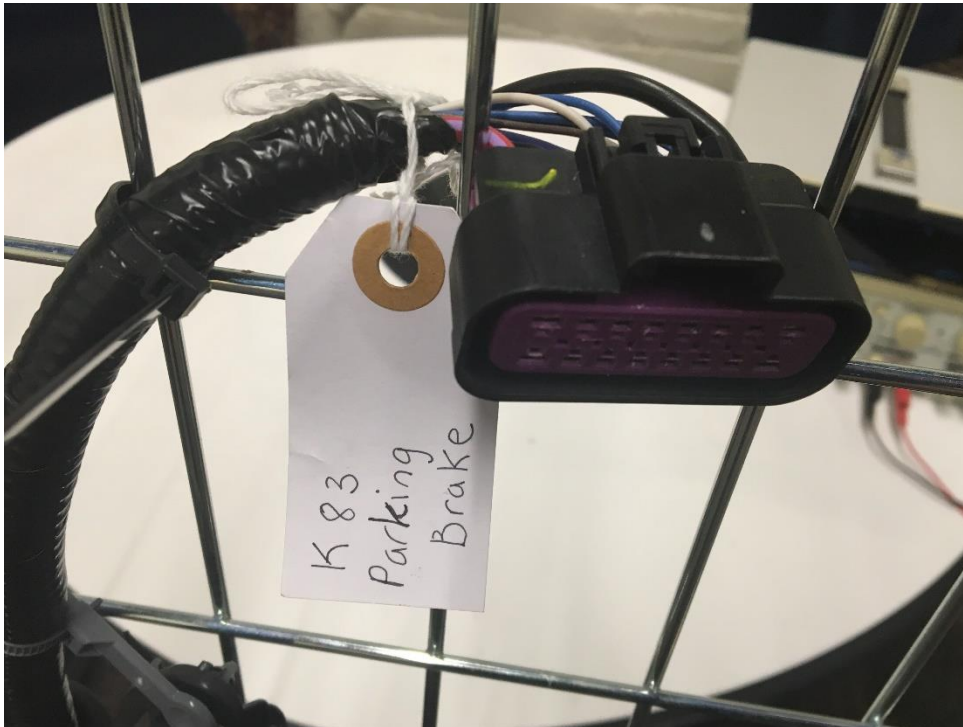
Figure 24: Connector on the 2015 Chevy Impala wiring harness. The connector has been marked by the previous MQP team with a paper tag that identifies it as the K83 connector that is used by the parking brake.
