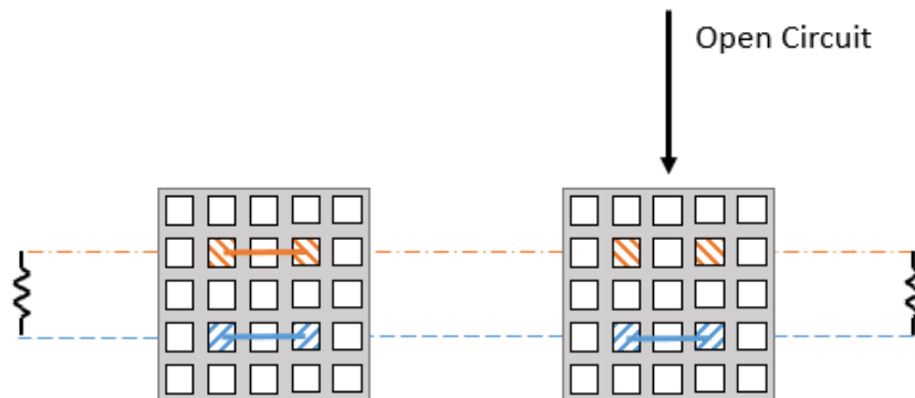
Figure 33: Example of a sort circuit when 2 pins on a connector are not bridged. The harness connector does not automatically bridge the gap between the two pins, and so it is up to the device connector to do so.
