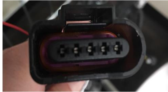
Figure 25: K43 Power Steering connector in the documentation for a 2014 Chevy impala and on the 2015 Harness. The documentation indicates a 10-pin layout in 2 rows of five, while the connector on the harness only has 5 pins in a single row.
