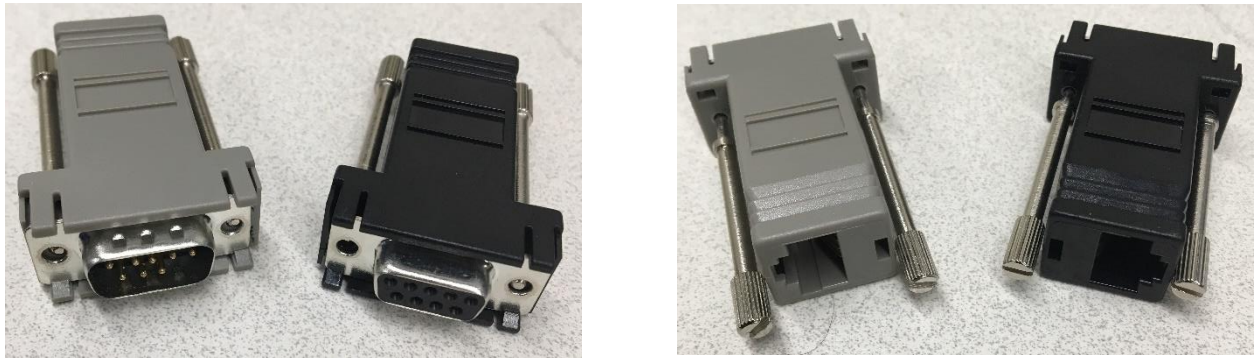
Figure 40: DB9 to CAT5 converters. Any CAT5 cable can be inserted to lengthen the distance between the harness connector and the ECU.
