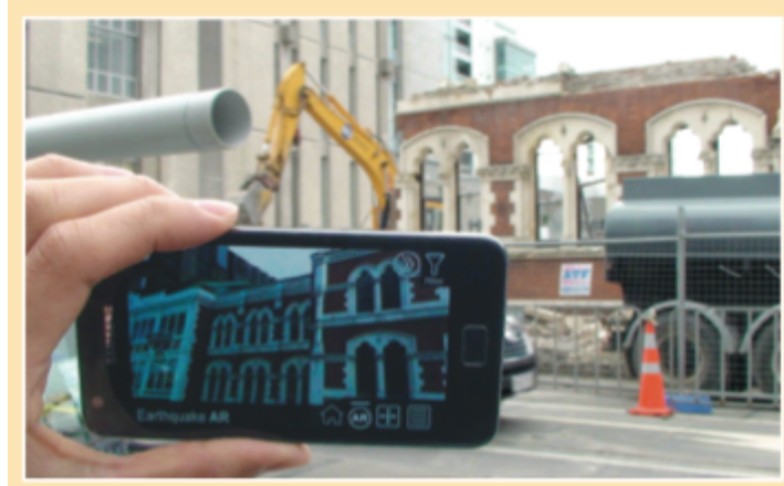
Figure 2. The CityViewAR application showing the history of earthquake-damaged Christchurch. The application uses the mobile phone's GPS and compass sensors to superimpose a virtual undamaged building on the site of the real building remains.
