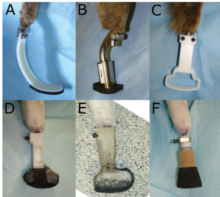
Figure 10: Images showing some different types of designs and materials used for transcutaneous parts of the ITAP implant. (A) Blade design made from carbon fiber; (B) metal concentric cylinders with a rubber insert; (C) rocker made from Derlin TM; (D) foam beds that are shock absorbing inserted in rubber that has Kevlar attached; (E) a deformable polymer design that is one-piece; (F) a multidirectional foot piece made with a Derlin TM shaft [31]
