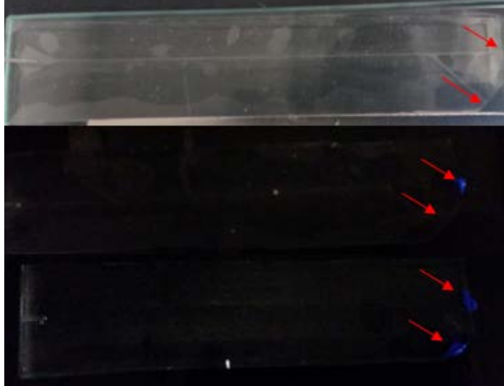
Figure 22: Chambers with luminol: healthy blood (middle) and infected blood (bottom), chamber at top used as reference for orientation. Red arrows indicated location of collection wells. Pictures taken with cell phone camera.
