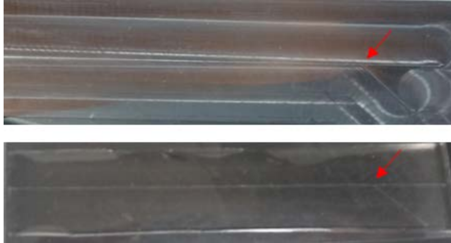
Figure 16: Milled mold (top) and PDMS chamber (bottom), approximately 127mm in length. Red arrow indicates where the chamber splits on both the negative and casted chamber
