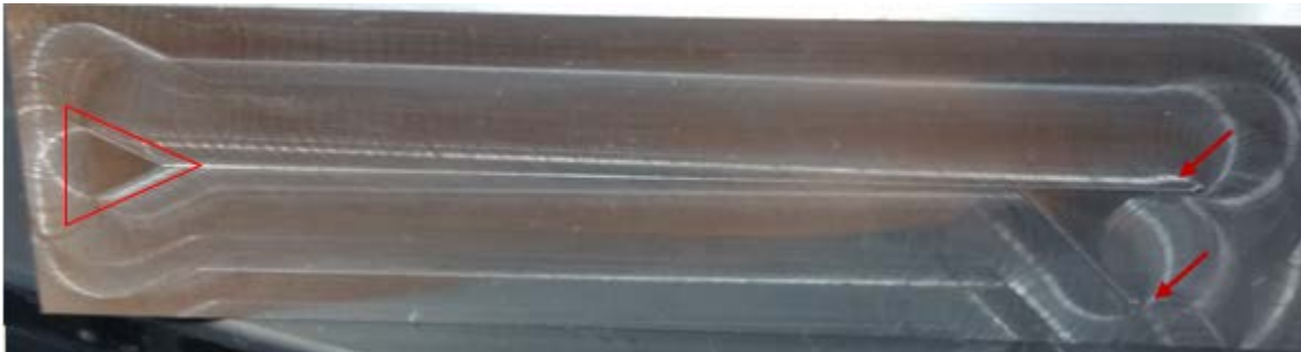
Figure 18: New chamber with larger entry port (red triangle), collection chambers indicated by red arrows.
