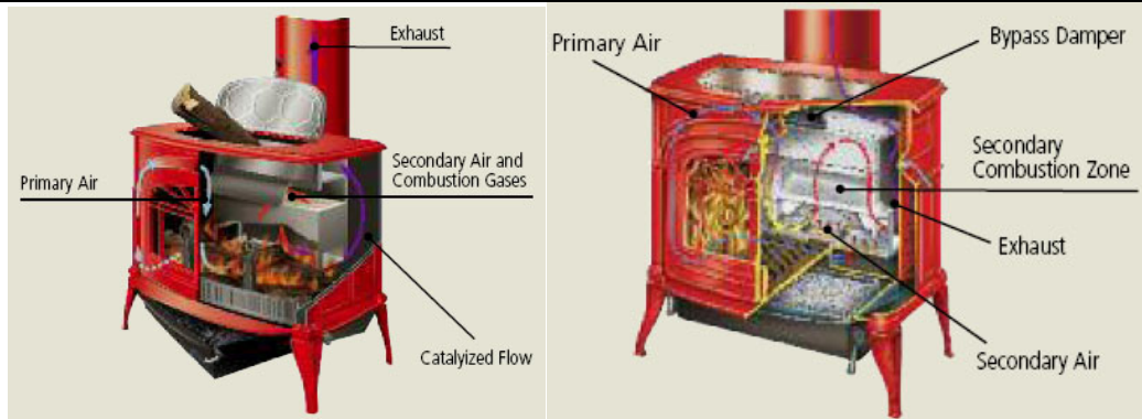
Figure 18: Non-Catalytic Wood stove (right), Catalytic Wood Stove (left) [20]
