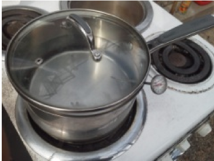
Figure 24: Thermometer, pot, and lid arrangement for experiment on range top
