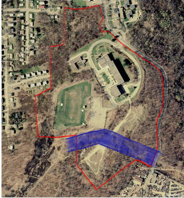
Figure 41: Existing Utility Lines and Easement
