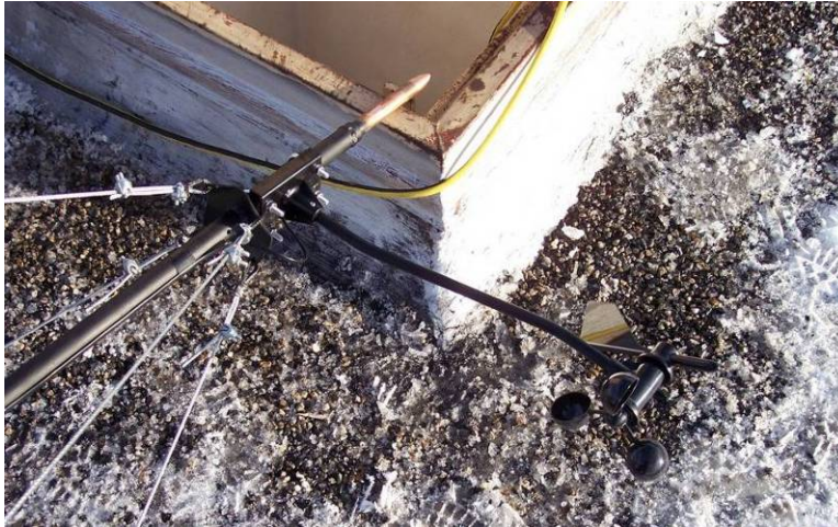
Figure 29: Copper Electrode and Weather Station Affixed
