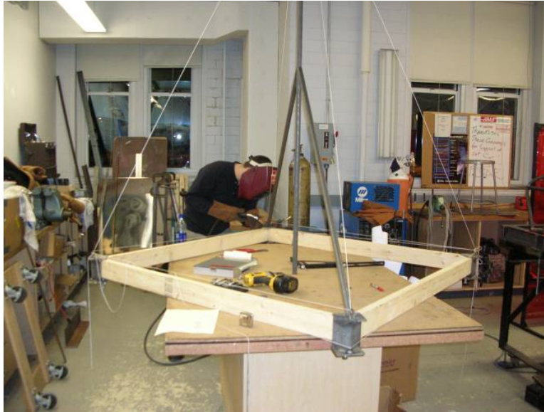
Figure 25: Wooden Jig Constructed, Corner Bracket Being Welded
