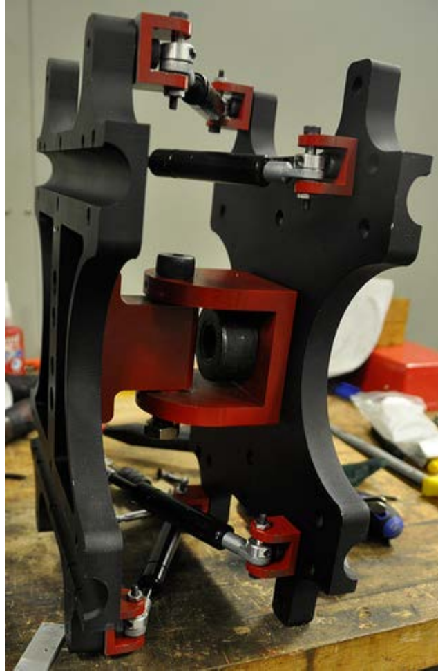
Figure 119 - Completed Body Joint
