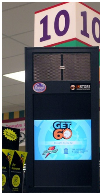
Figure 6- A hypersonic sound device has been placed in this mall display (ATCSD.com)
