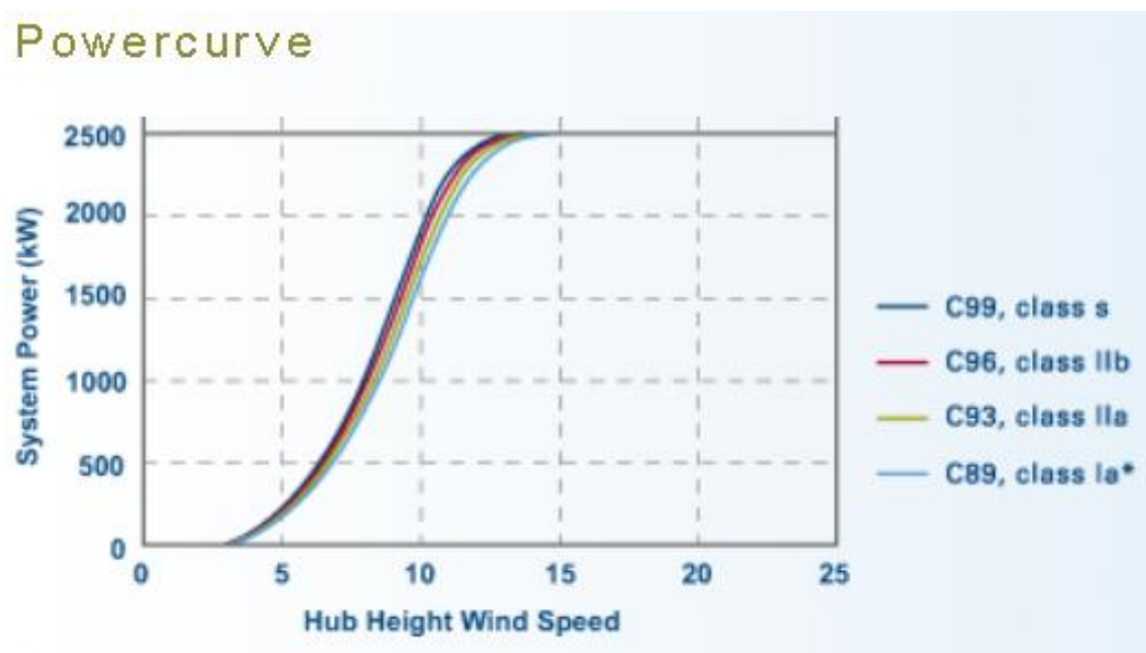
FIGURE 7: CLIPPER LIBERTY TURBINE POWER CURVE [CLIPPER WINDPOWER]
