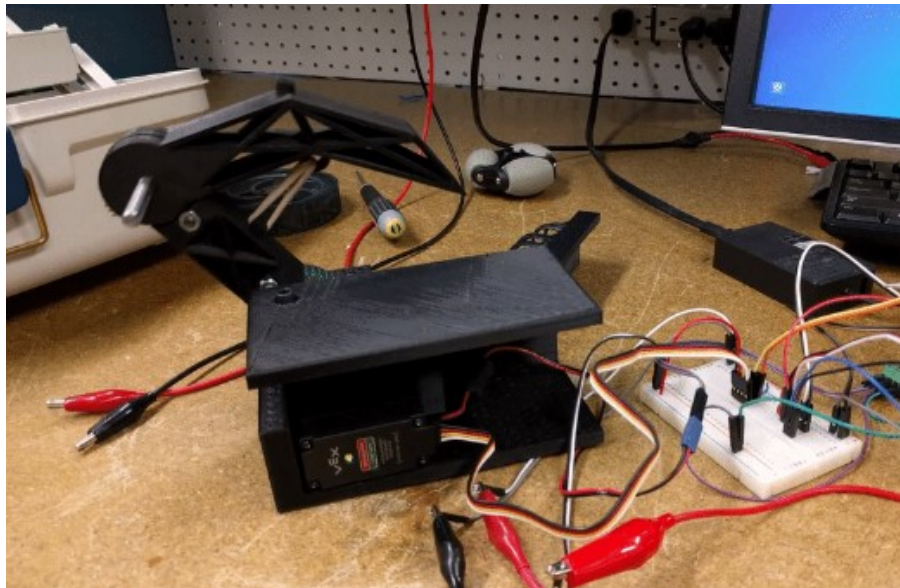
Figure 24: Leg testing configuration
