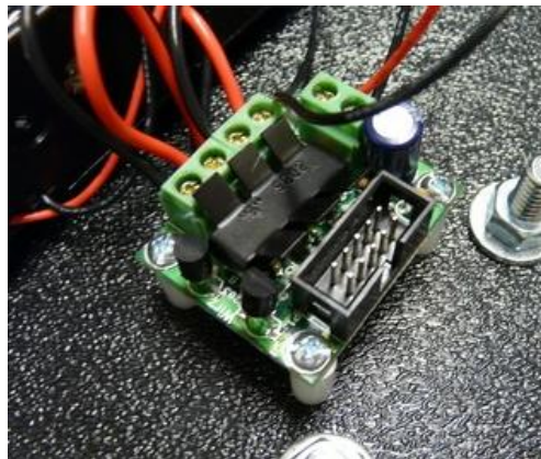
Figure 12 - WIRZ #203 Motor Controller Mounted to Robot Deck
