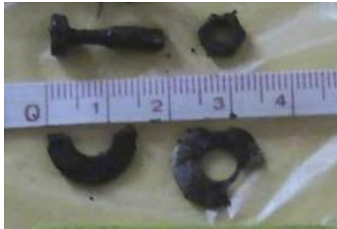
Figure 26: Corroded bolt, nut, and washers
