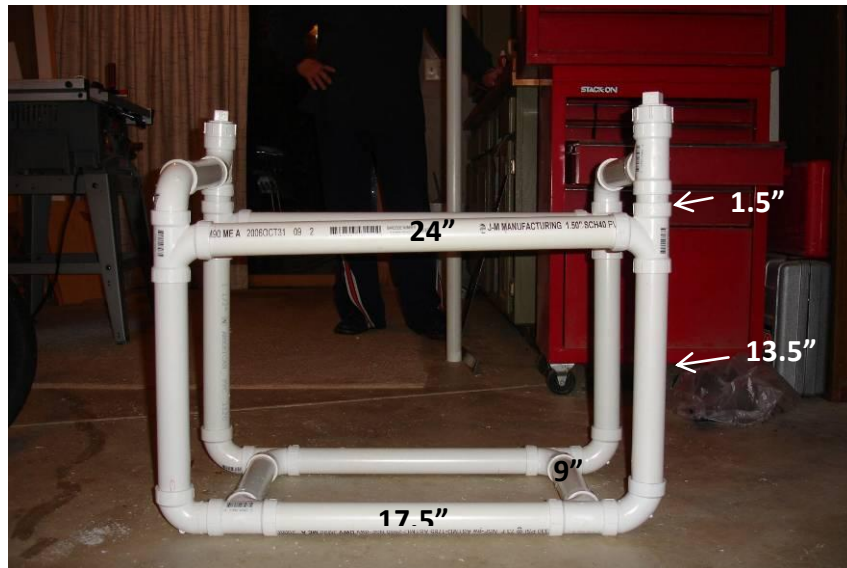
Figure 14: Dimensions for Connecticut apparatus frame
