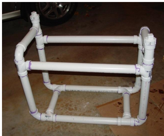
Figure 11: Assembled frame for Connecticut apparatus
