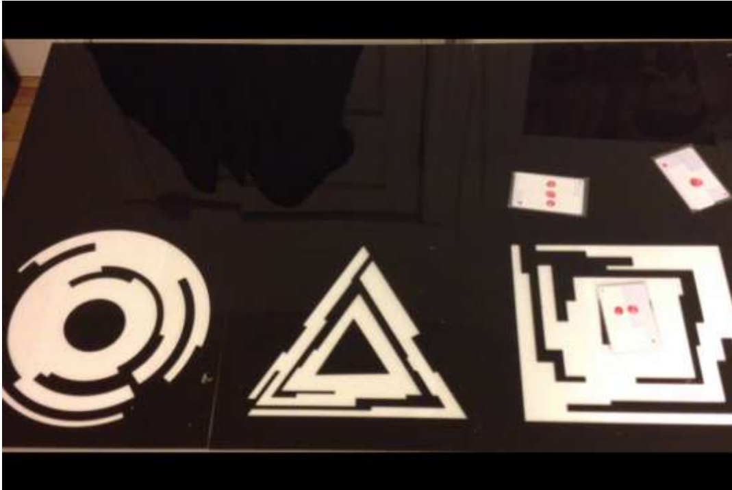
Figure 73: The laser cut acrylic pieces. The RFID tags can be seen to the right.
