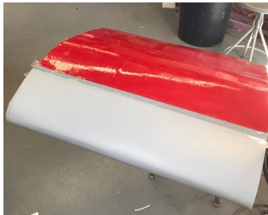
Figure 59: Wing leading edge smoothed using Polyethylene sheet.
