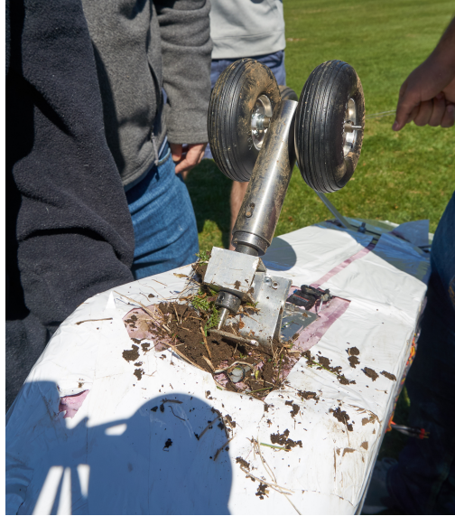
Figure 61: Damaged front landing gear after flight test.
