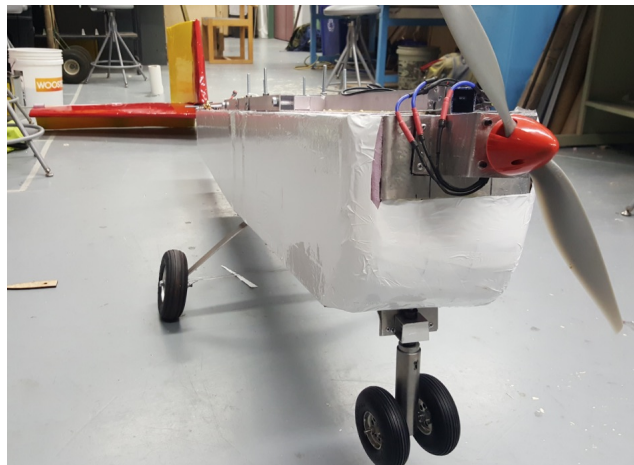
Figure 52: Completed nose with propulsion equipment installed.
