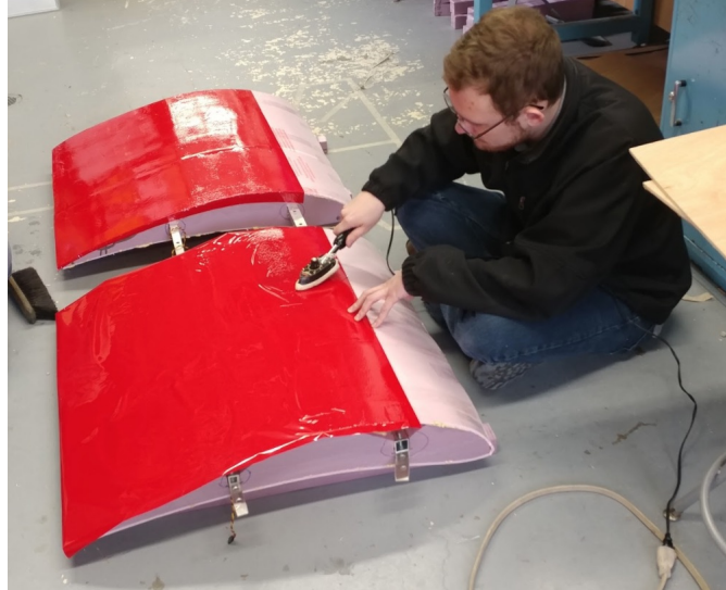
Figure 47: Heat sealing the Monokote skin to the wing.
