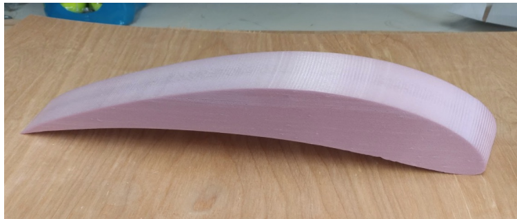
Figure 44: Completed foam rib fabricated by hot wire cutting.
