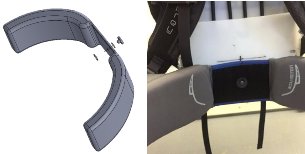
Figure 29: (Left) Exploded view of the pivoting unit assembly. (Right) Image of the assembled unit.
