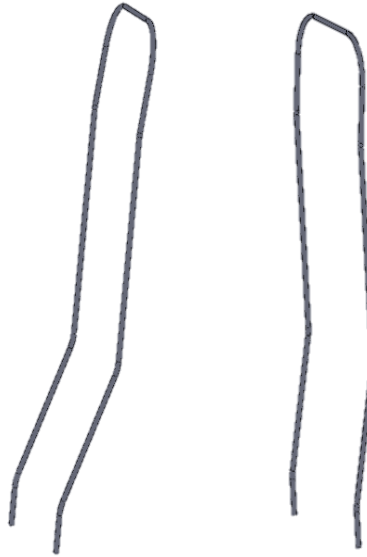
Figure 23: (Left) 7075 frame with more pronounced prongs at the end. (Right) 6061 frame with less pronounced prongs at the end
