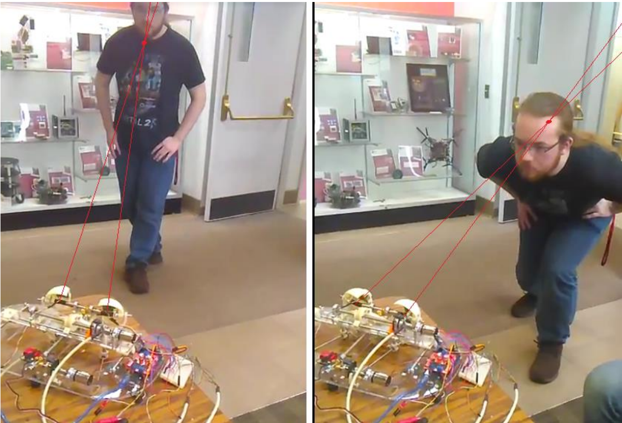
Figure 58: HSV System tracking a face
