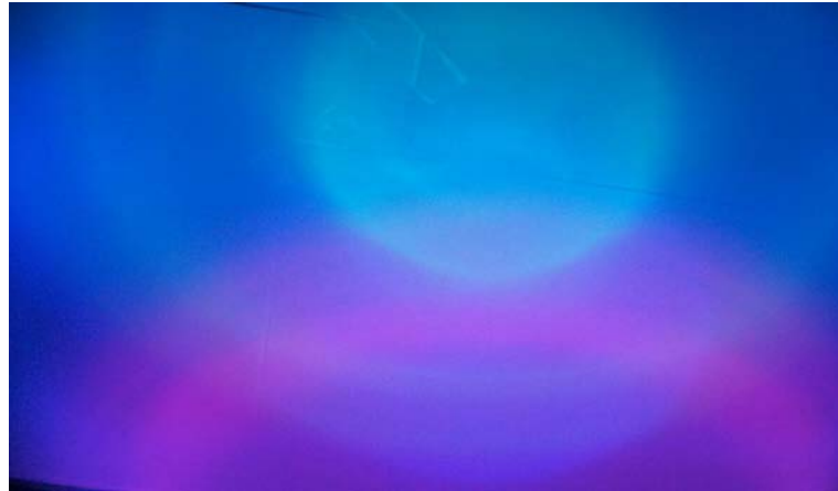
Figure 4–2: Poor Color Blending from RBA Single Lens LED4.1.2 Microcontroller
