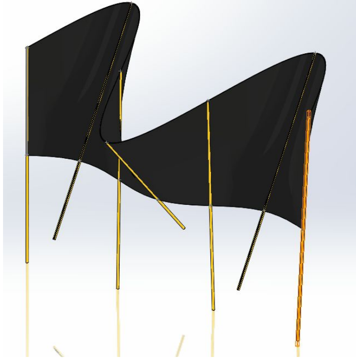
Figure 12: SolidWorks Model of Fin with Masts
