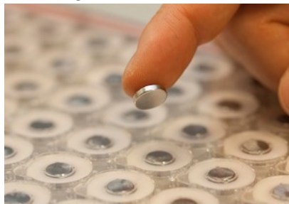
Figure 20: FingerFlux electromagnet array [47]
