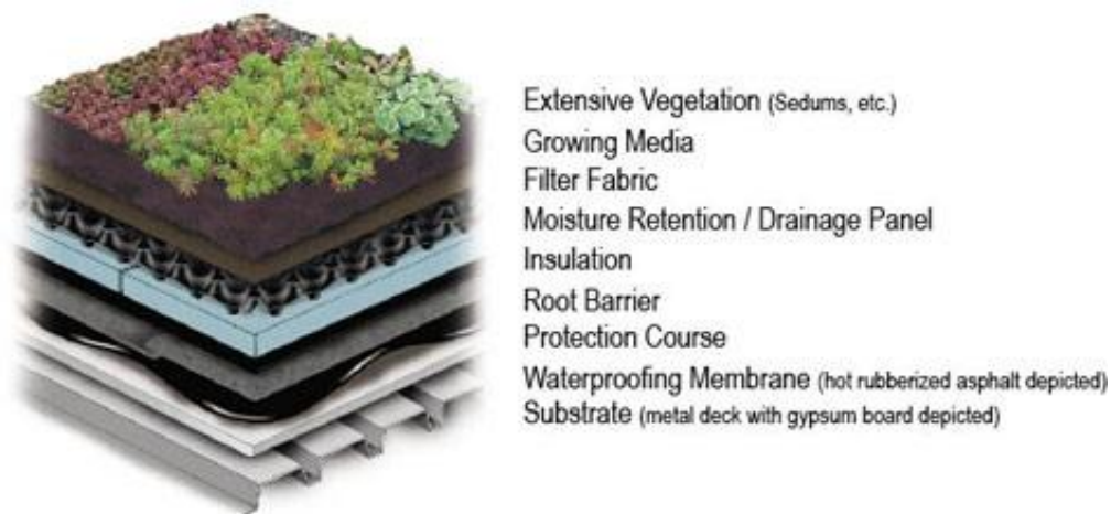
Figure 8 - Extensive Roof Section (Miller, 2011)
