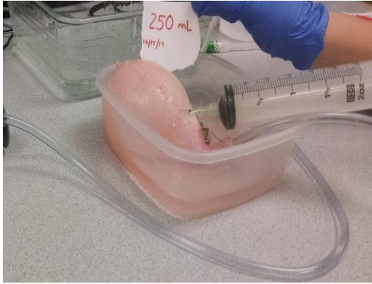
Figure 46: Bladder at 250mL and corresponding pressure-volume plot
