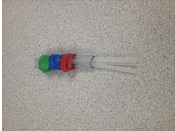
Figure 29 Three Tiered Balloon catheter that fills balloons individually
