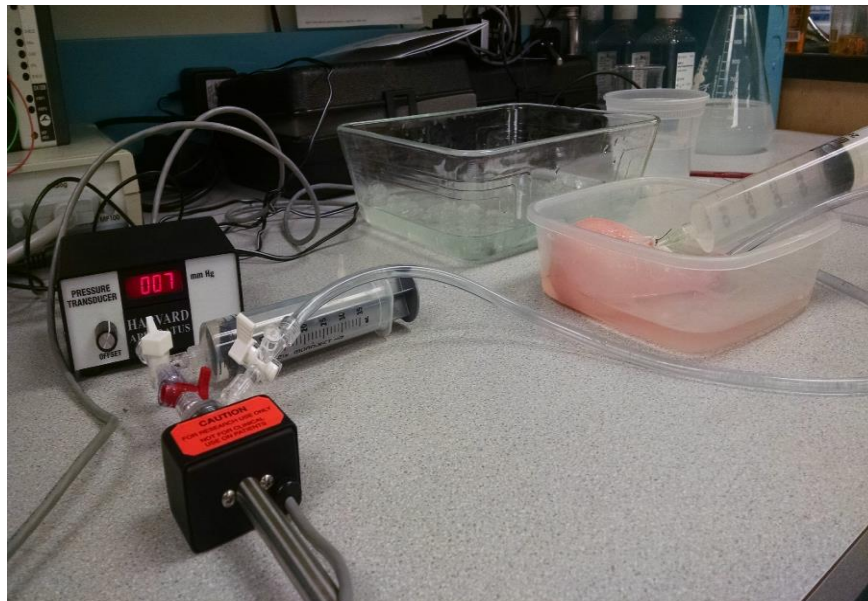
Figure 41: Pressure Test Setup for the Bladder
