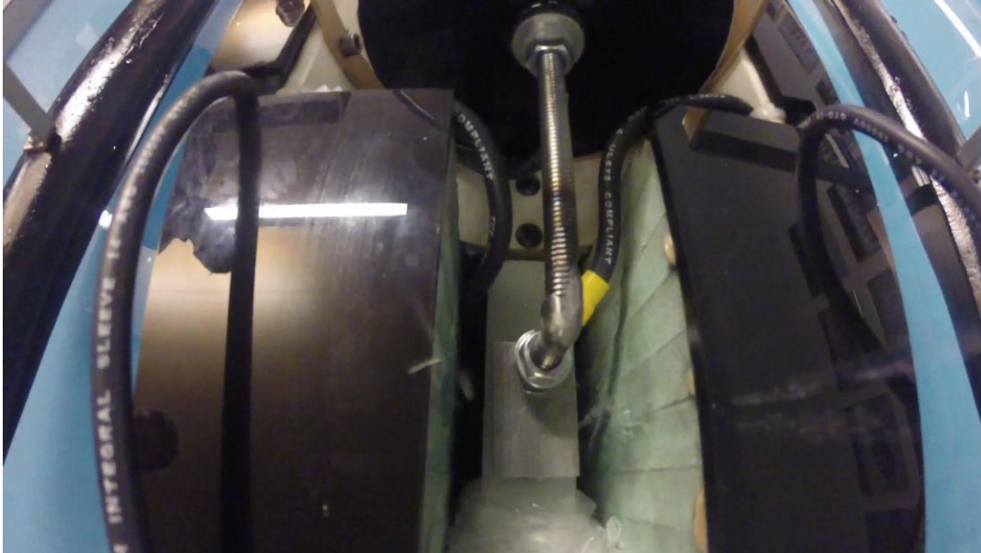
Figure 40: Frame from GoPro onboard video with water splashes from chamber leaks.
