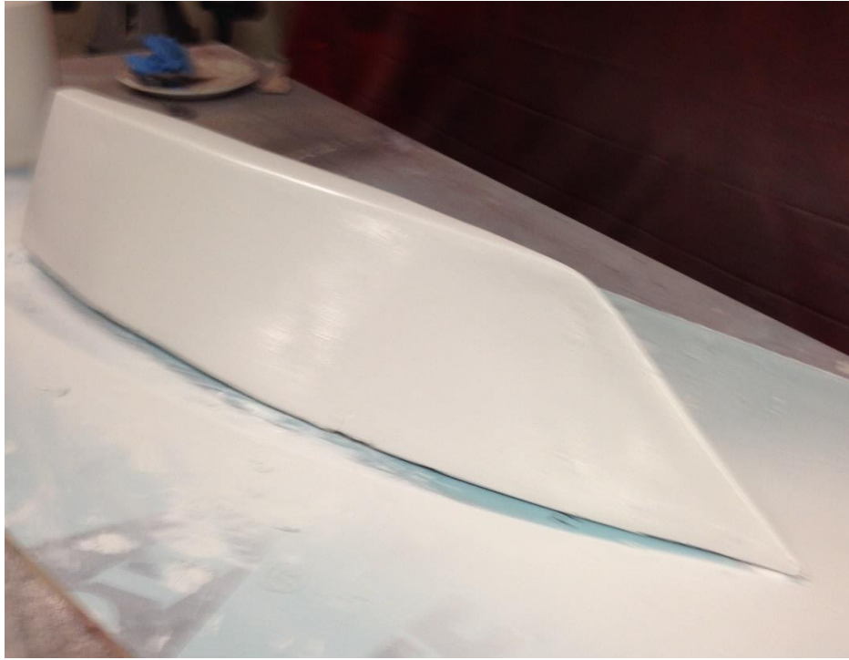
Figure 41: Vaka hull after application of Gel-Coat.
