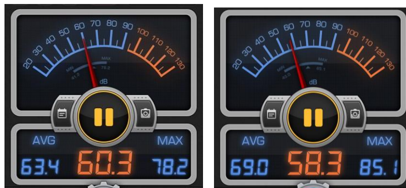
Figure 28: Decibel readings with Acoustic Foam (left) and without (right)
