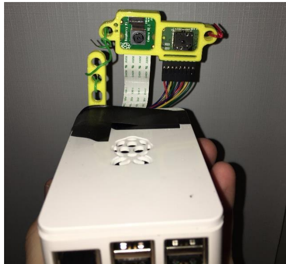
Figure 29: Pi Camera (left) and Lepton Module (right) in 3D Printed Frame
