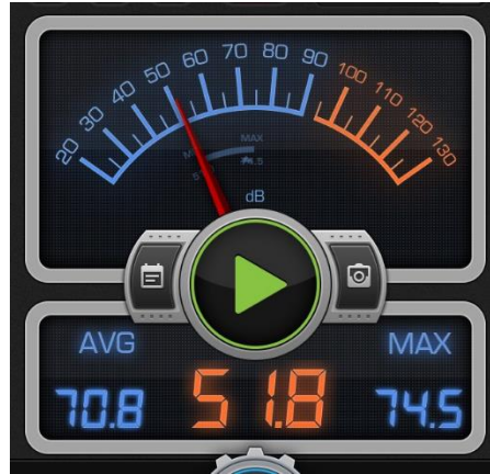
Figure 44: Decibel Reading of Speaker at 300Hz from 1 Meter Away
