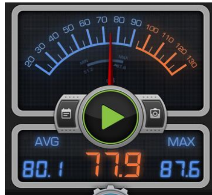
Figure 45: Decibel Reading of Speaker at 300Hz from 1 Meter Away (with housing)
