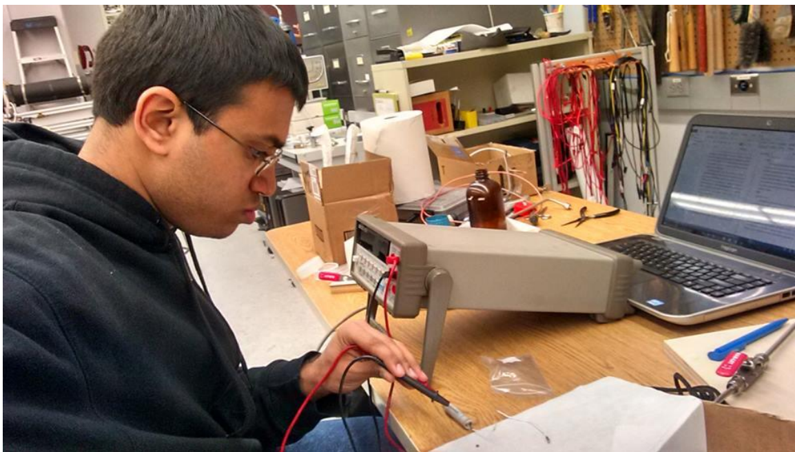
Figure 16: Checking connection of electrodes to bus lines.
