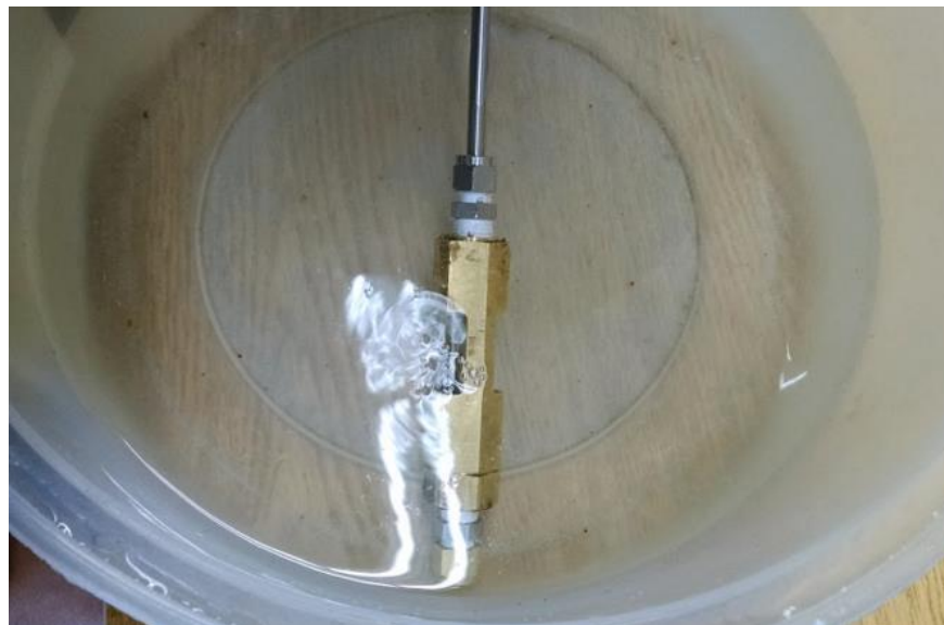
Figure 30: Underwater leak testing method.
