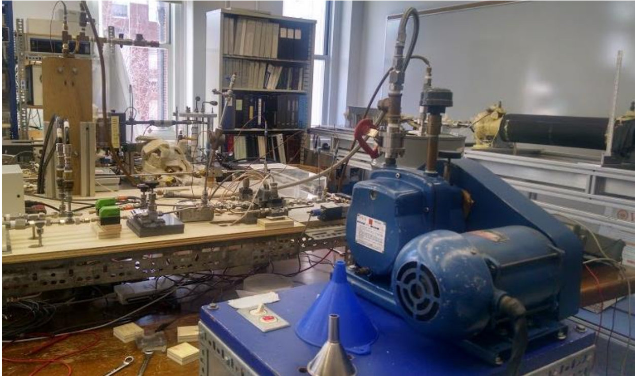
Figure 32: Genco HYVAC 7 pulling a vacuum.
