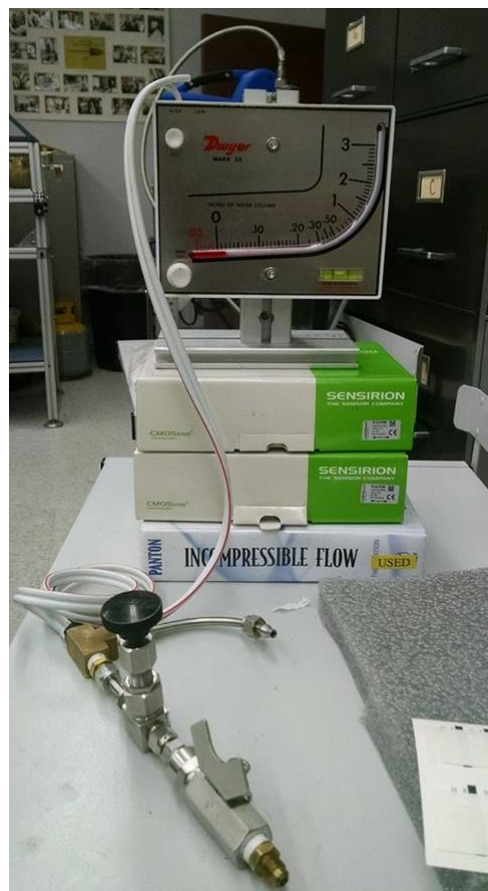
Figure 26: Differential pressure transducer calibration apparatus.
