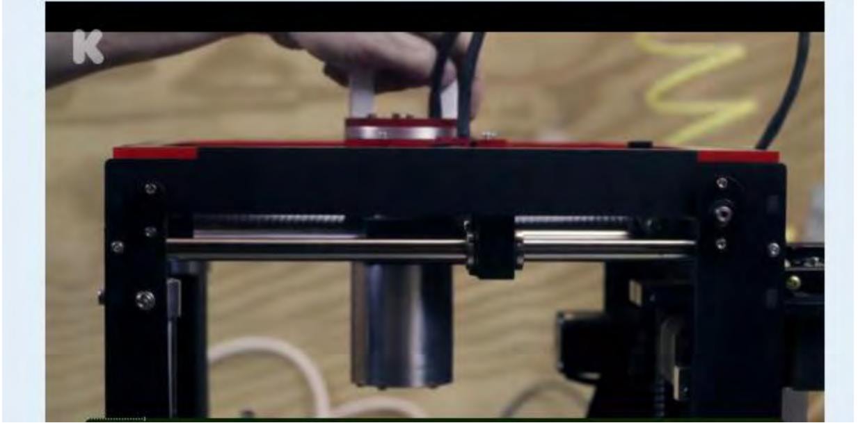
Figure 16. BoXZY being loaded with its 2 watt laser (Alec. 2012)
