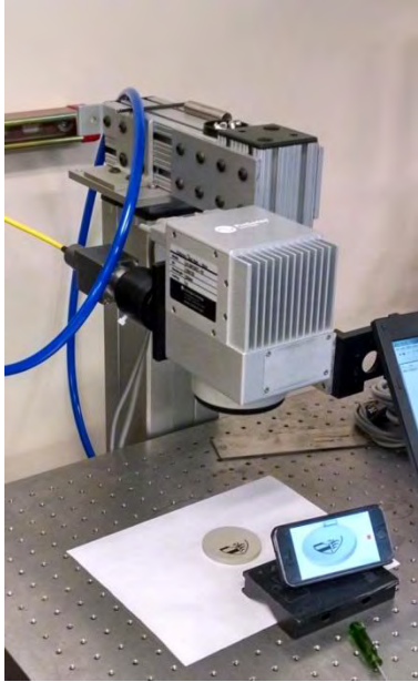
Figure 26. A Galvo scanner, making a test mark at IPG Photonics
