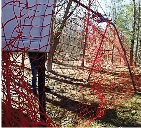
Figure 13: Test 3, modified B-net with the elastic zone
