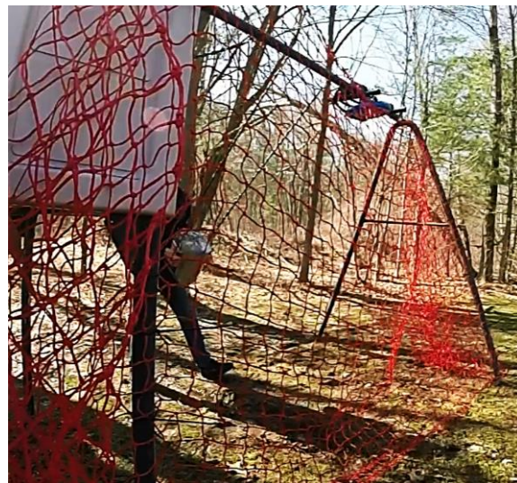
Figure 12: Test 2, a loosely hung net with about 0.25 meters of slack
