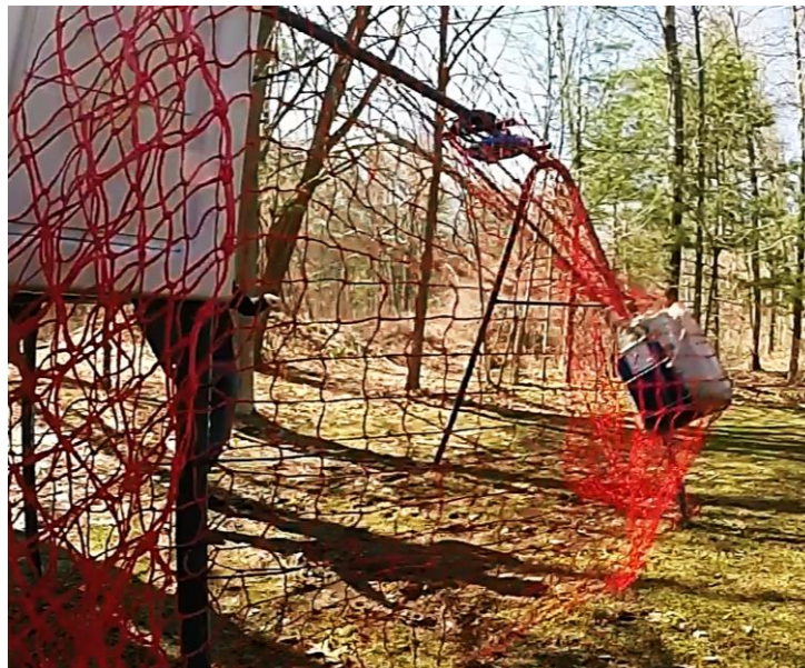
Figure 15: Maximum net stretch when hung loosely
