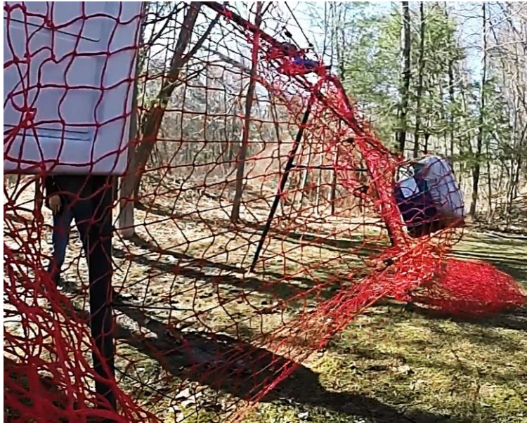
Figure 16: Maximum net stretch with modified B-net
