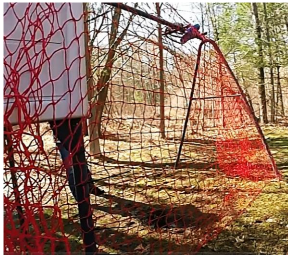
Figure 11: Test 1, a tightly hung net similar to how the current generation of B-nets is set-up
