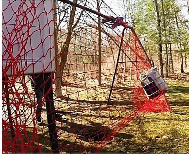
Figure 14: Maximum net stretch when hung tightly
