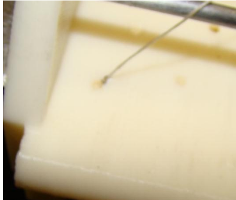
Figure 63: Wear in Guidance Channels
