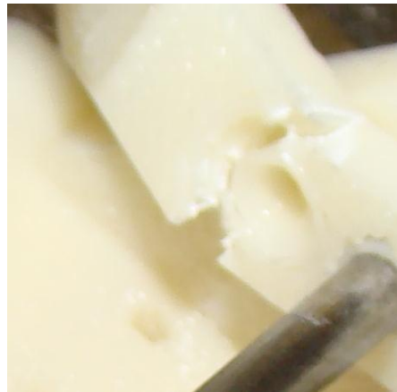
Figure 60: Crack in V Bracket Around Screw Hole
