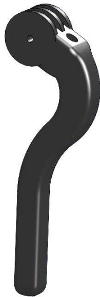
Figure 19: Second Generation Lower Leg
