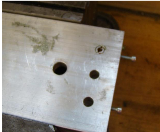
Figure 42: Drilling Shaft Hole
