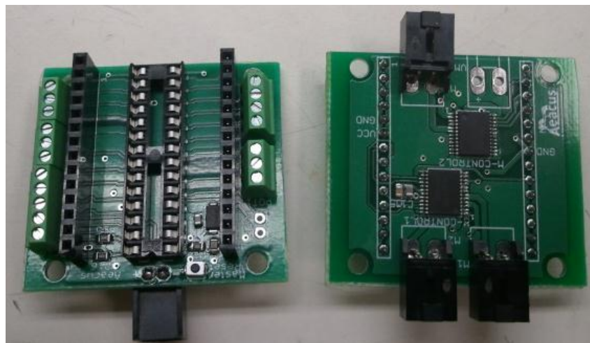
Figure 68: Leg Controller Separated
