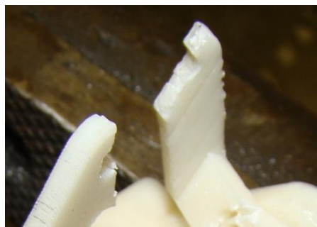
Figure 59: Crack in V Bracket Around Axle Hole
