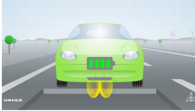
Figure 56 - Electric car charging via induction loops in the road 244
