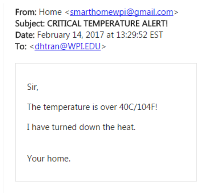
Figure 56: Example of severe temperature warning sent from server.
