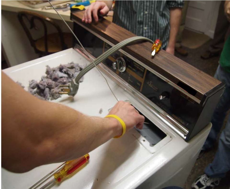
Figure C- 6: Process of Removing Lint from Clothes Dryer
