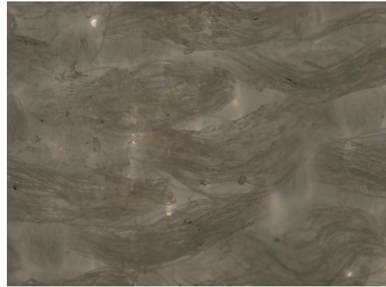
Figure 13: Woven polyester graft, outer view (5X)
