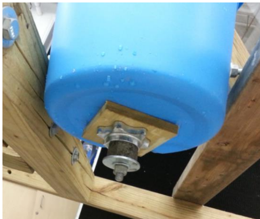
Figure 20 - The weight underneath the tipping bucket
