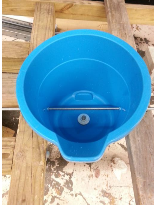
Figure 19 – Inside of the tipping bucket mechanism
