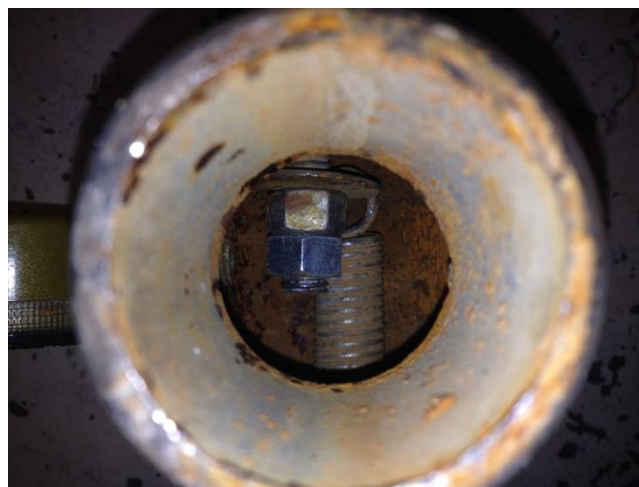
Figure 14 - The spring and rod within the pressure simulator pipe
