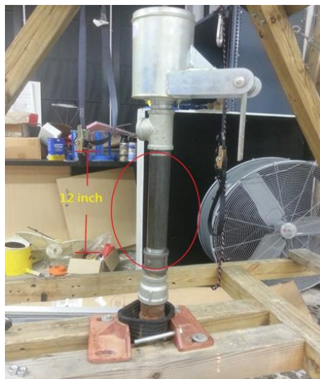
Figure 17 - Extended and raised water-pump piping
