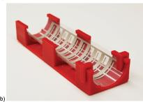
Figure 10: Macro-scale pump (a) wrapped cylindrically (b) flexed in semi-cylindrical configuration.
