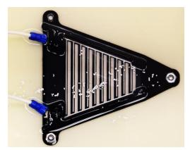
Figure 19: Nozzle pump in flat configuration
