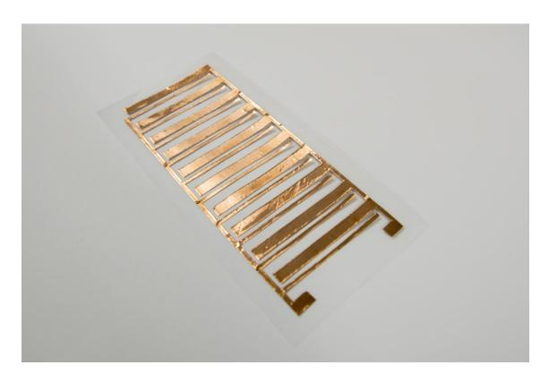
Figure 5: Copper tape macro-scale pump.
