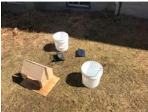
Figure 39. Solar Panel Water Fountain
