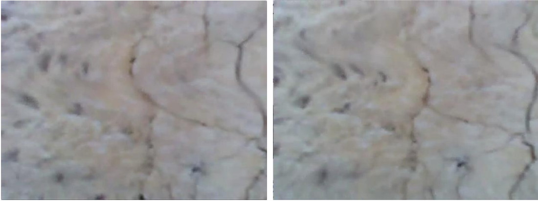
Figure 50: Camera images with the engine on, when the camera is simply taped to the bottom of the plane.
