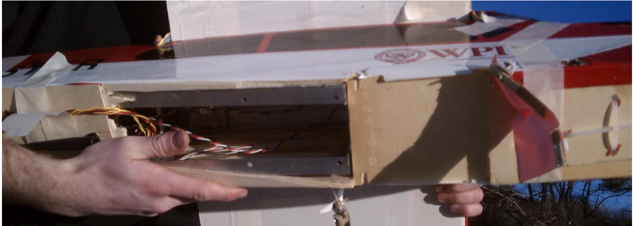
Figure 43: What remains of the bottom of Robin's fuselage after its February 18th crash. Notice how it is missing its landing gear and wing strut attachment points. The Aluminum frame prevented further damage.
