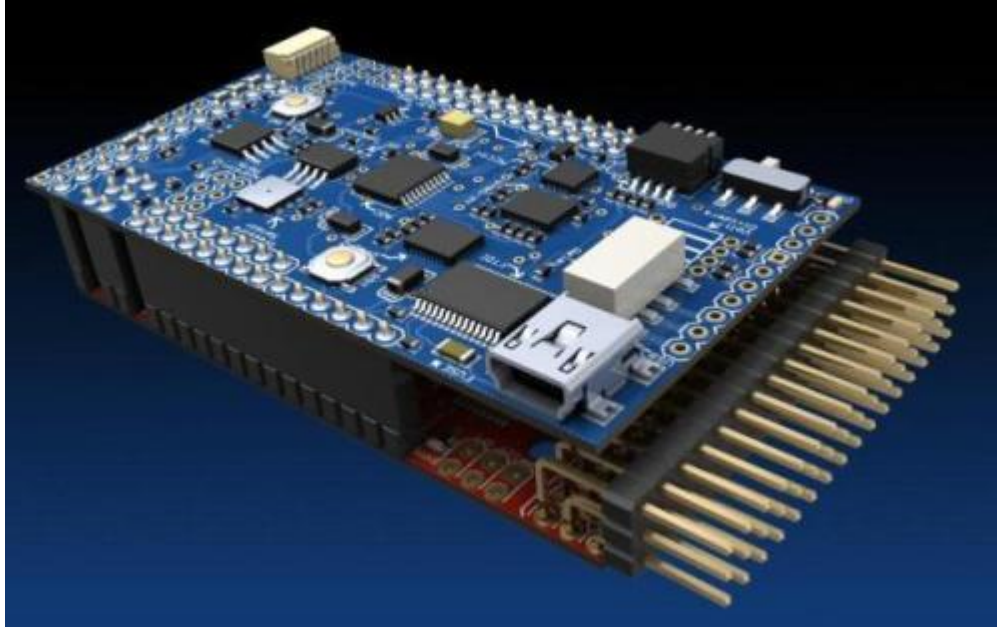
Figure 53: Ardupilot is an open source autopilot solution featuring arduinos.
