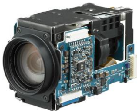
Figure 24 Sony color block camera that we will put in the planes
