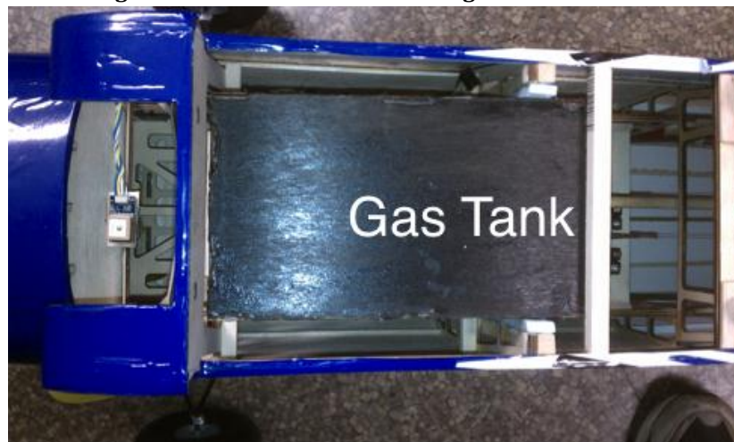
Figure 30: The fuel tank chamber in place in the body
