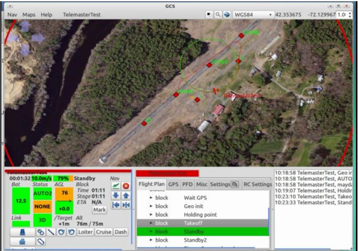
Figure 81: Screen capture of the ground control station during a launch simulation
