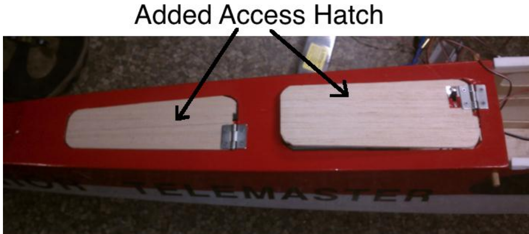
Figure 21: Robin with back hatches installed
