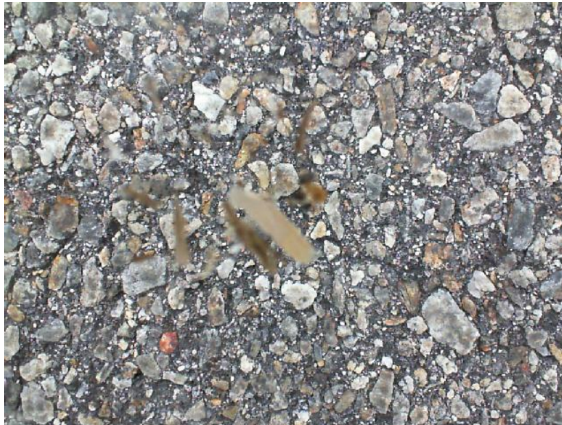
Figure 49: Camera image with the engine off, when the camera is mounted properly with vibration dampening
