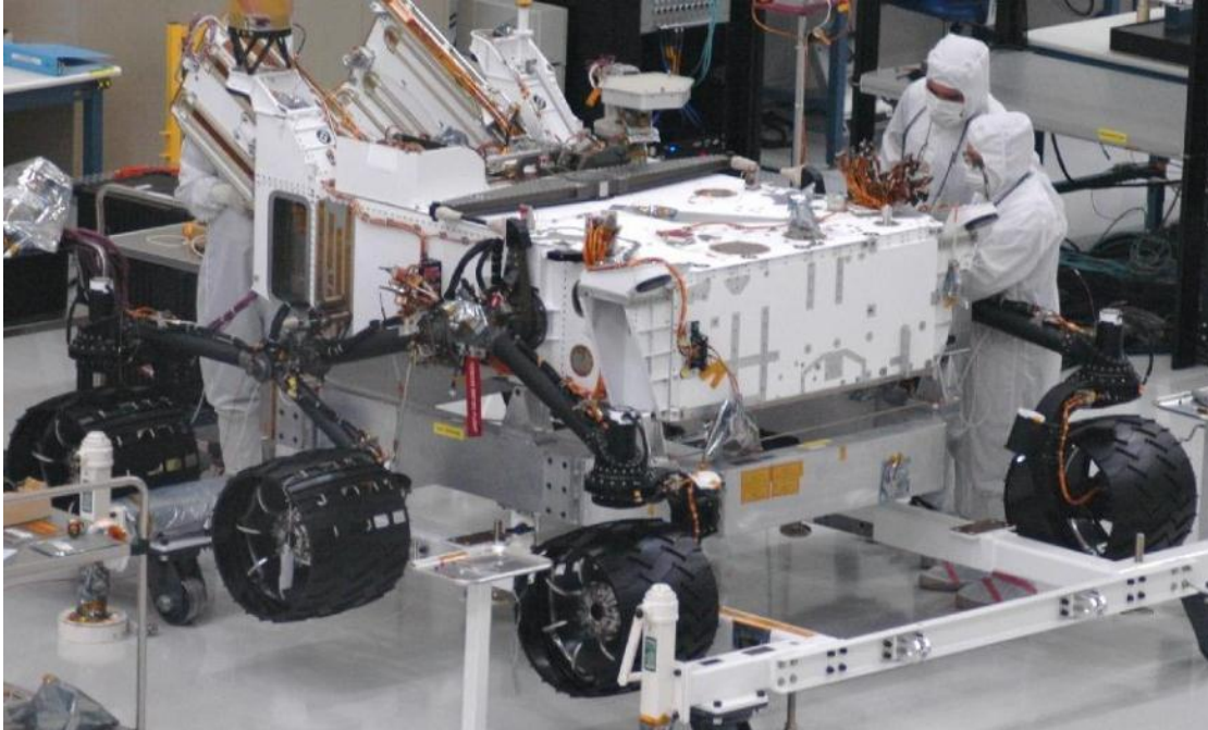
Figure 5: Mars Science Laboratory chassis showing suspension and wheels.
