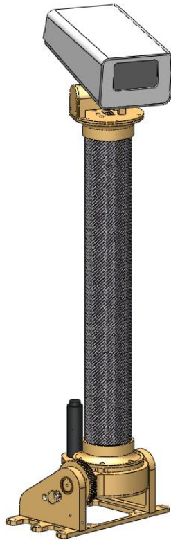
Figure 37: Design of Deployable Camera Payload
