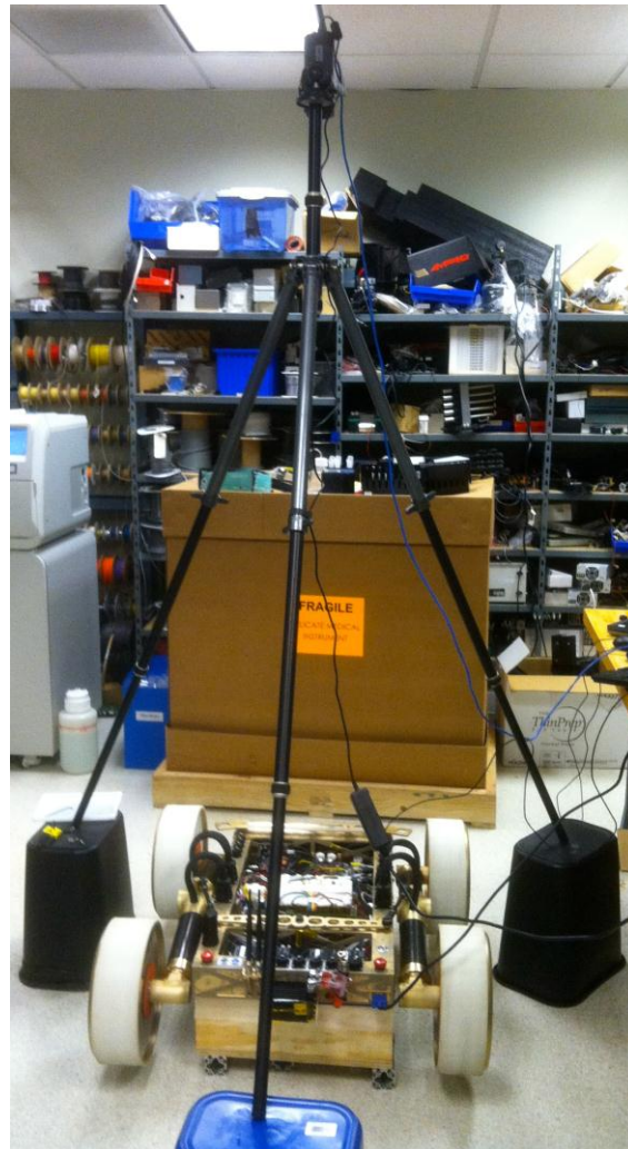
Figure 49: Experimental Setup for System Level Thermal Monitoring Testing
