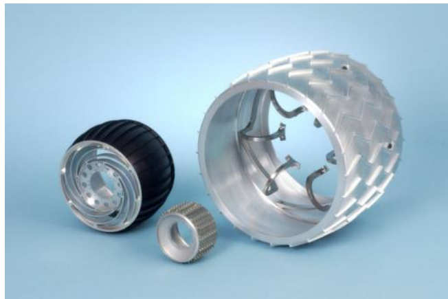
Figure 4 : (L-R) MER, Sojourner, and MSL wheels
