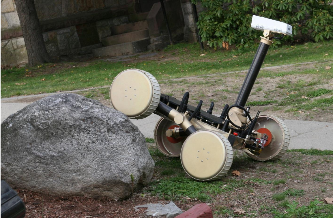
Figure 57: Camera Payload Deployed while Traversing Large Rock
