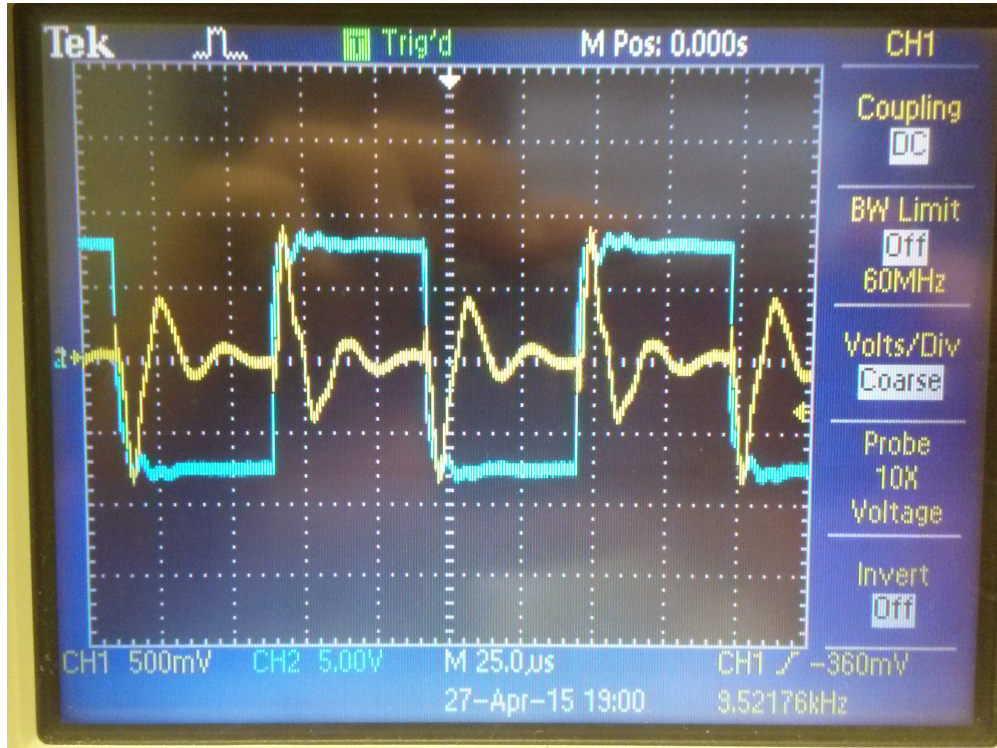
Figure 6.8: Graphs of the output signal to the transmitter coil (Blue) and the voltage drop across a 10\Omega output resistor (Yellow)
