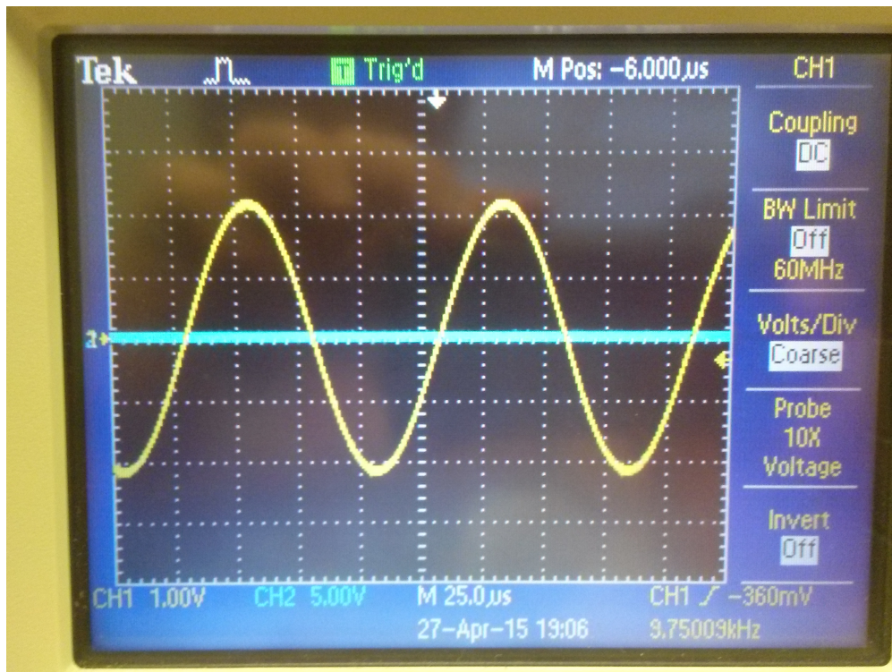
Figure 6.9: Graph of the output voltage from receiver coil across 10\Omega load resistor
