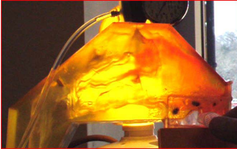
Figure 15: Flow through post-turbineotomy nasal cavity at 45 mmHg
