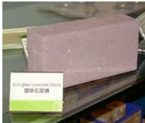
Figure 7. Laputa's glass paving block on display at Coca-Cola's Sha Tin Bottling Plant.
