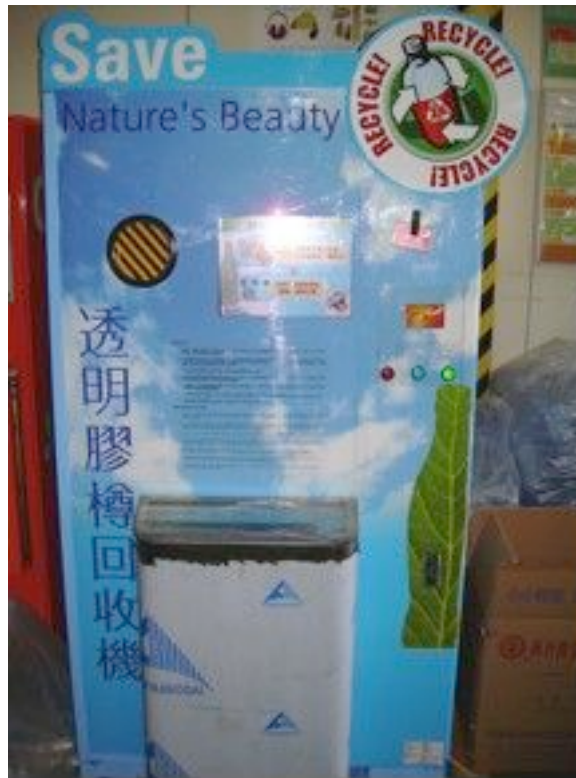
Figure 9. Coca-Cola's PET (polyethylene terephthalate) bottle “reverse” vending machine.
