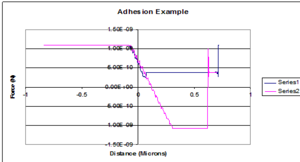
Figure 25: Example of Adhesion: The attractive forces applied to the probe are so great that they will bend the cantilever to a critical force where the cantilever will break or the bond between the tip and sample will, skewing any data obtained.
