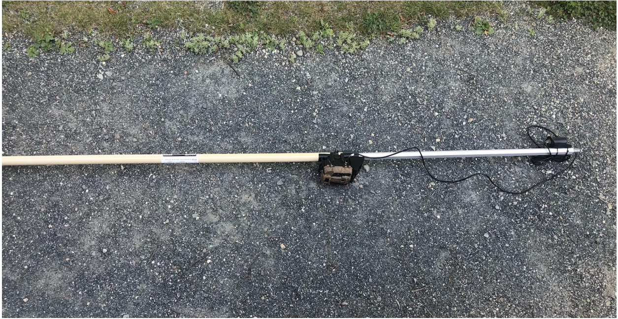
Figure 9: Camera Setup with Long Range Boosting Antenna
