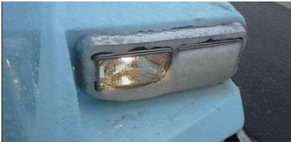
Figure 8 Snow accumulation on LED headlight [1]
